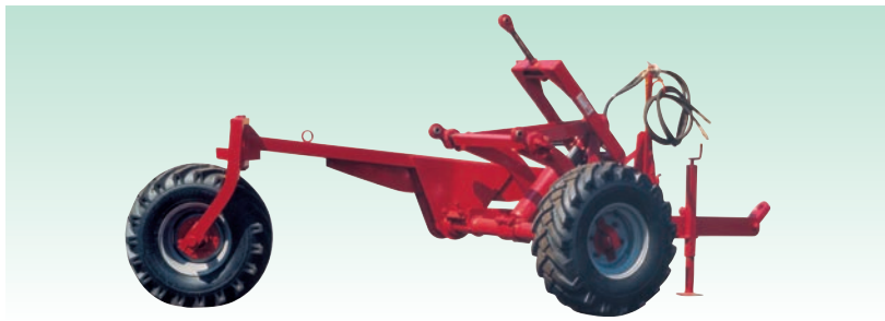
Trainati: carrello con braccio; cingoli o ruote fuori solco. Trailed: carrier with arm, tracks or wheels outside the furrow.
